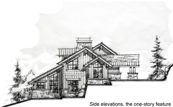
Side elevations, the one-story feature on the rear of the home must be at least one-third of the overall width of the home.
