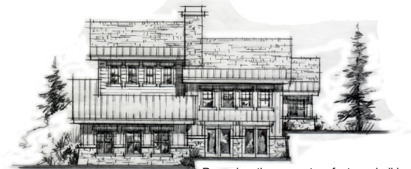
Rear elevation, one-story feature shall be at least two-thirds of the width of the overall width of the entire structure.
